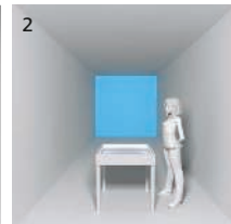
A lighting design that uses low-glare LED strip luminaires that are hidden around the edge of the display cabinet, making them and their reflections almost invisible to customers. This also provides a much better uniformity of illumination.
