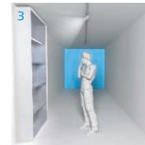
By positioning LED strip luminaires on the lower edge of shelves, all shelves are optimally illuminated. LED light sources are perfect for this because they emit negligible amounts of heat, allowing them to be positioned very close to even fragile items.
