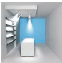
A boutique style payment counter using statement suspended luminaires to highlight and illuminate the counter, and accent lighting spotlights to provide suitable vertical illumination of the display behind.
